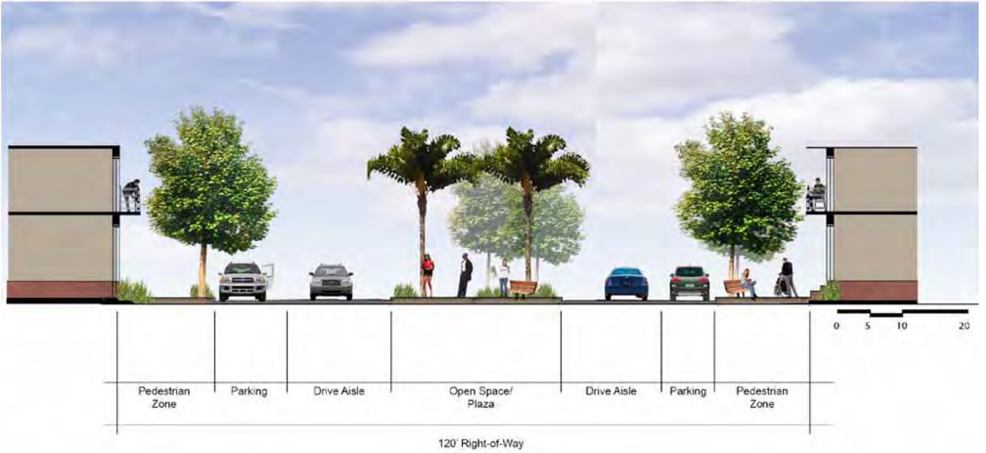
Image 13: Dimensions of a 120-foot right-of-way. Created by CPAT member, Claire Hempel, AICP
